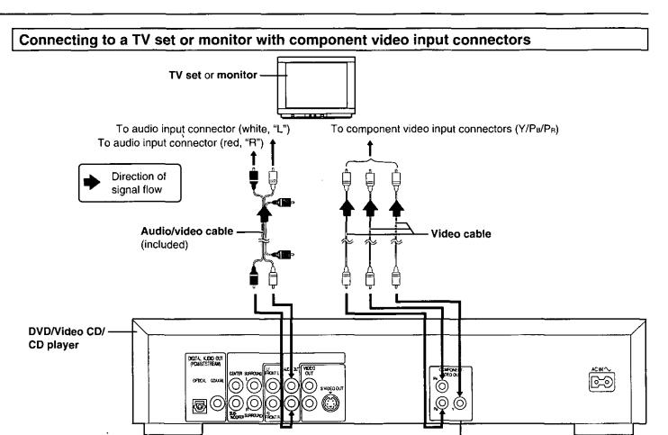
The component video output connector outputs the color difference signals (P<sub>B</sub>/P<sub>B</sub>) and luminance signal (Y) separately in order to achieve high fidelity in reproducing colors.
